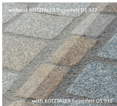
**KÖTZTALER Fugenfest DS 932** is an environmentally friendly 2-component polymer dispersion for consolidating sand-filled joints. The sand that has been swept into the joint is soaked with **DS 932** to bind it. This results in joints that are robust, non-slip and resistant to frost or weathering.
