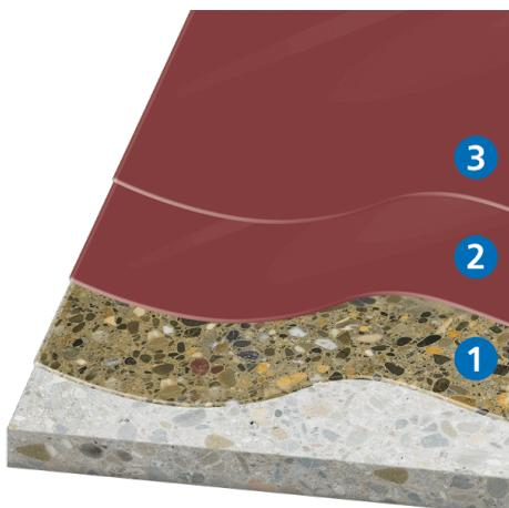
3. Second sealing layer with **KLB-SYSTEM EPOXID EP 740 E**
