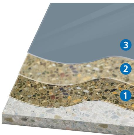
3. Top coat **KLB-SYSTEM EPOXID EP 282 WHG** - optional: injecting structured granulate **Strukturgranulat RQX 9/RQX 10**
